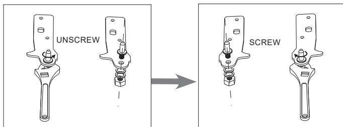
6. Refit the bracket fitting the botton hinge pin. Replace both adjustable feet.
