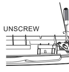
4. Remove the screws and bottom hinge. Then remove the adjustable feet fromboth side.
