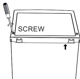
11. With the door closed, check that the door is aligned horizontally and vertically and that the seals are closed on all sides before
