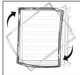
8. Place the door back on. Ensure the door is aligned horizontally and vertically so that the seals are closed on all sides before
