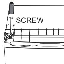
9. Connect the terminals onto the display board, then put top cover back.
