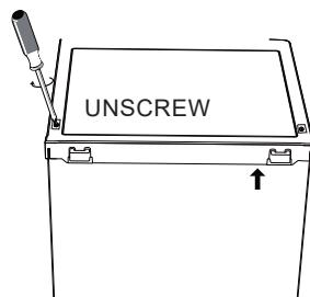
2. Carefully lift the top cover 5CM away from the freezer, then pull out the terminal. Then removethe top cover away
