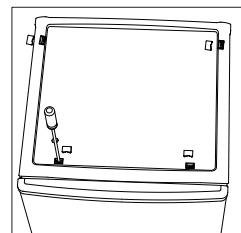
2. Unscrew and remove the hinge. Then lift lower door and place it on a soft pad to avoid scratch.
