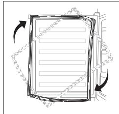
9. Make the middle hinge reverse the direction  $180^\circ$ , then transfer it to the left property position. Place the lower door back on. Make the middle hinge pin in the upper hole of the lower door, then tight the bolts.
